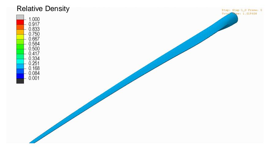
Optimal distribution of material for blade load case identified
